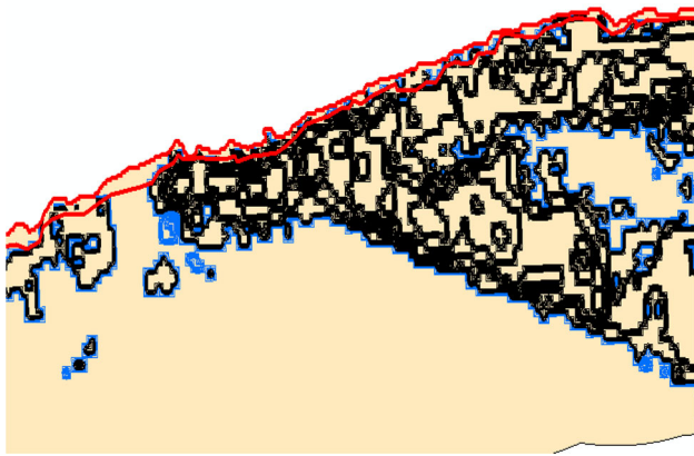
Fig. 12 A sample for the barrier line (red) separating low-lying areas (blue) near the coasts from high ones (black) or far away low-lying areas (WGS84)
