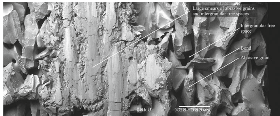
Fig. 3 Micrograph of visible smear of intergranular space of grinding wheel active surface after grinding Titanium Grade 2 ® obtained by JEOL JSM 5500LV scanning electron microscope produced by JEOL Ltd. ( U_a = 20 kV, Mag. \times 50 )
