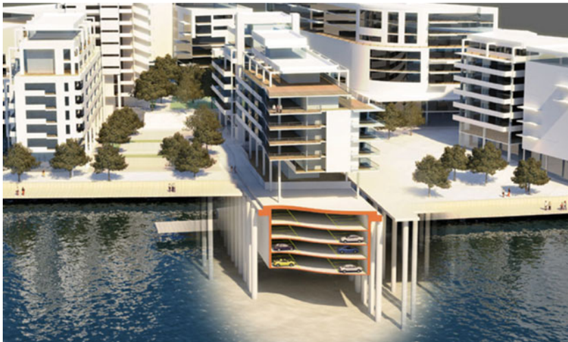
Fig. 9 A model section showing how the prefabricated concrete caissons provide large submerged parking areas in four levels
