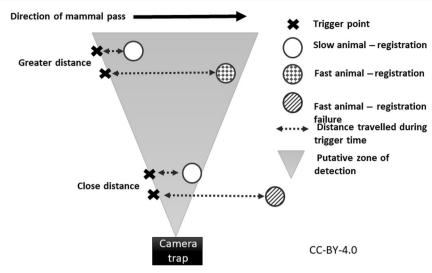
**Fig. 8** Hypothesized mechanism showing how distance to camera-trap (CT) can interact with animal speed to influence registration probability. Registration probability is positively affected by distance due to the larger
