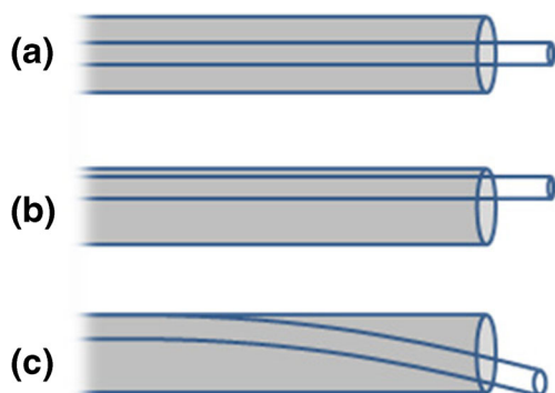
Figure 1. Positioning of the solvent capillary in the laboratory-built desorption electrospray ionization (DESI) sprayer. Ideally, the fused-silica solvent capillary should be concentric with the gas capillary (a), resulting in rotational symmetry and an even distribution of the nebulization gas flow. Because of the flexibility of the fused silica, however, it is usually off-center (b) or bent and protruding at an angle (c)
