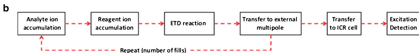
Figure 1. (a) Conceptual layout for the 21 T FT-ICR mass spectrometer with which all experiments were conducted. This system features a dual cell linear ion trap, a multipole storage device, a dynamically harmonized cell, and a 21 tesla actively shielded superconducting magnet. (b) Experimental event sequence, showing how multiple fill experiments were conducted
