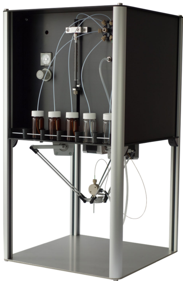
Figure 1. Open-source software and hardware device for matrix deposition. The design was optimized to allow a fully automated process, including priming and cleaning. Protocols can be downloaded to the device from any source, fostering co-development between labs
