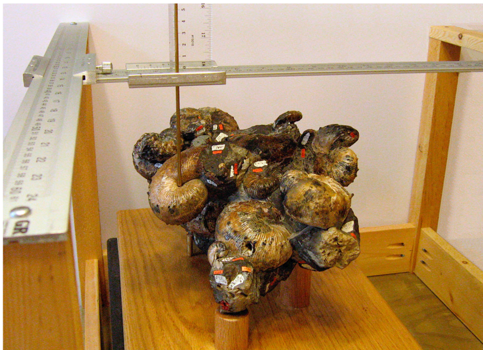
Fig. 2 The large 3-D framework with long (610 mm) built-in vernier calipers designed to measure the orientation and position of the ammonites in the concretion. The main accumulation of ammonites (the “sculpture”) is visible in the foreground. The view is toward the southeast end of the sculpture and slightly above. The 3-D system is mounted on a wooden frame and consists of two calipers that have had their normal jaws removed from the vernier sliding bars. The rail or ruler of the second, movable one ( Y axis or width, at the top of the photo from left to right ) is attached (with drilled and tapped screws) to the sliding bar of the first, fixed one ( X axis, or length, at the left side
