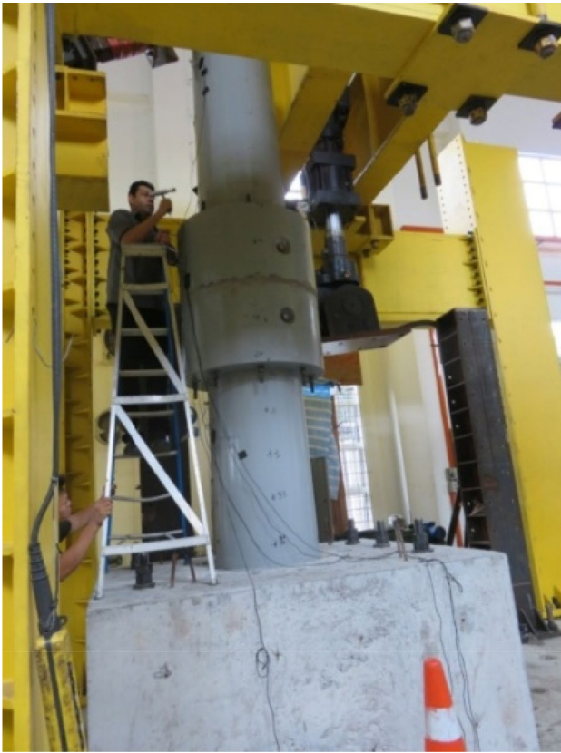
Fig. 21 Knocking bolted foundation segment after adding epoxy
