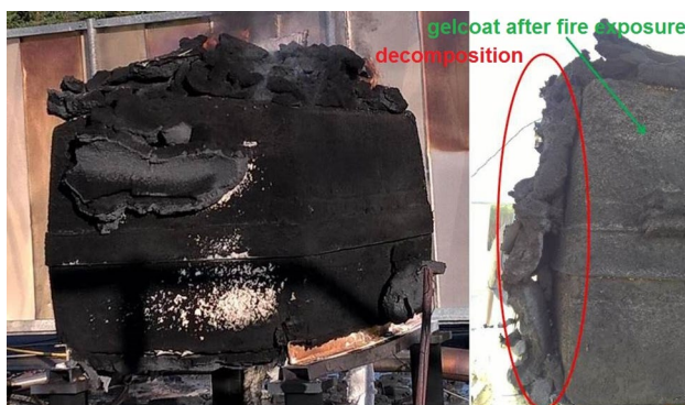
Fig. 7 Heat-related decomposition of the fire protective thermoplastic foil applied on the outer tank surface
