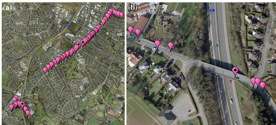
Fig. 15 Vehicle position coordinates logged using Leica GS14 on test route 2 a overview, b on bridge
