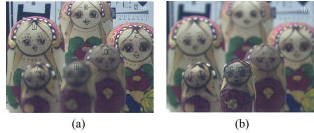
Fig. 3 Far focused and near focused images: (a) negative LC lens optical power and (b) positive LC lens optical power.
