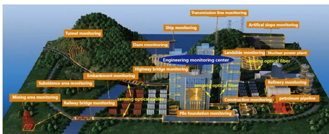
Fig. 1 Distributed fiber geo-aware system concept diagram (the yellow highlight line in the figure is sensing fiber).
