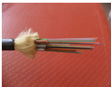
Fig. 4 Picture of 72 optical fibers with the type SMF-28.
