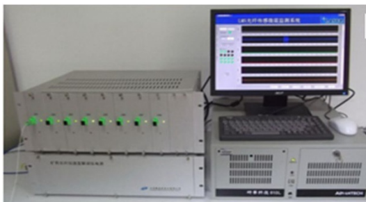
Fig. 7 Micro-seismic demodulator and data processor.
