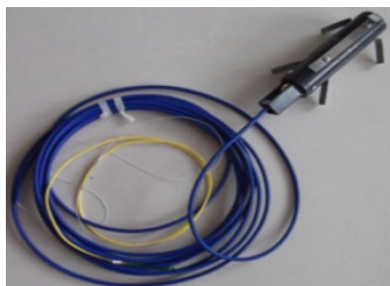
Fig. 6 Improved FBG geophone.
