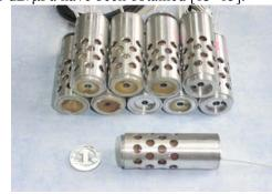
Fig. 14 Fiber seismic hydrophones.
