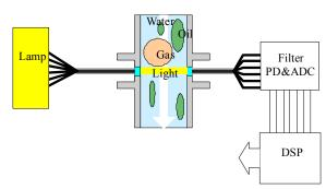
Fig. 8 Principle of the down well spectrometer.
