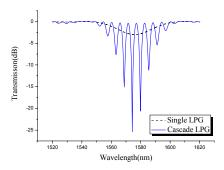
Fig. 3 Output spectrum of cascaded LFPGs.
