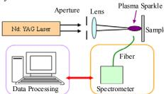
Fig. 10 Setup of LIBS system.
