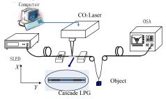
Fig. 1 Setup of LPFG fabrication.
