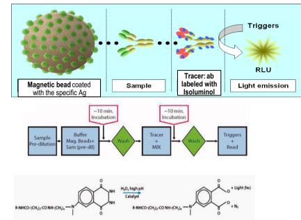
Chemical reaction of Assay scheme the light emission
