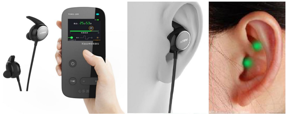
Fig. 3 Baseline medications of patients in active (left) and control (right) groups. Ta-VNS device TVNS-100 ® . Left, programmable stimulation device and ear electrode; middle, placement of ear electrode in the ear conch; right, the double stimulation points of the ear electrode in the ear conch
