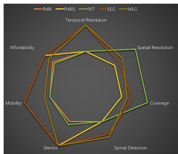
Fig. 1 Common neuroimaging techniques for assessing pain. This chart only represents the high and low rankings of various technologies, not the exact value. Temporal resolution: compared with other technologies, EEG and MEG have higher time resolution. Spatial resolution: fMRI and PET undoubtedly have the highest spatial resolution. Coverage: fMRI and PET provide detection of all regions of the whole brain, whereas other techniques usually cannot detect the prefrontal lobe and cerebellum. Signal detection: EEG and MEG directly provide neuronal activity, whereas other techniques detect it indirectly. Silence: fMRI and PET produce high noise in pain assessment, whereas fNIRS, EEG, and MEG are silent recording techniques. Mobility: the high mobility of fNIRS and EEG can be used for bedside monitoring, whereas other technologies do not do this due to the limitation of mobility. Affordability: compared with fNIRS and EEG, fMRI and PET are costly, followed by MEG
