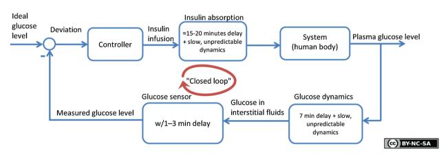
Fig. 2 Illustration of an artificial pancreas based on the double subcutaneous approach, including sources of delay. Reproduced with permission from [101]
