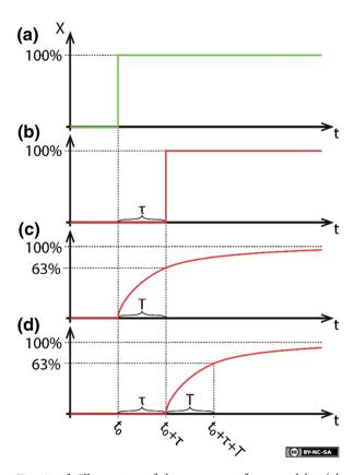
**Fig. 1a-d** Illustration of the concepts of a time delay  $(\tau)$  and a time constant (T). The system stimulus is shown in **a**, while the other figures illustrate the output from a system that presents **b** a time delay, **c** a time constant, and **d** both. This figure is licensed for publication under a Creative Commons BY-NC-SA 4.0 license
