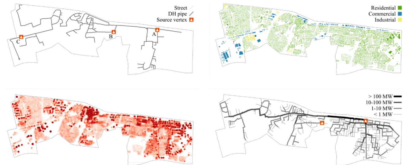
Fig. 4 District heating expansion planning in Munich: reference plan ( top left ) and optimization result ( bottom right ), derived from building stock ( top right ) and its estimated heat demand ( bottom left ) (Dorfner and Hamacher 2014)
