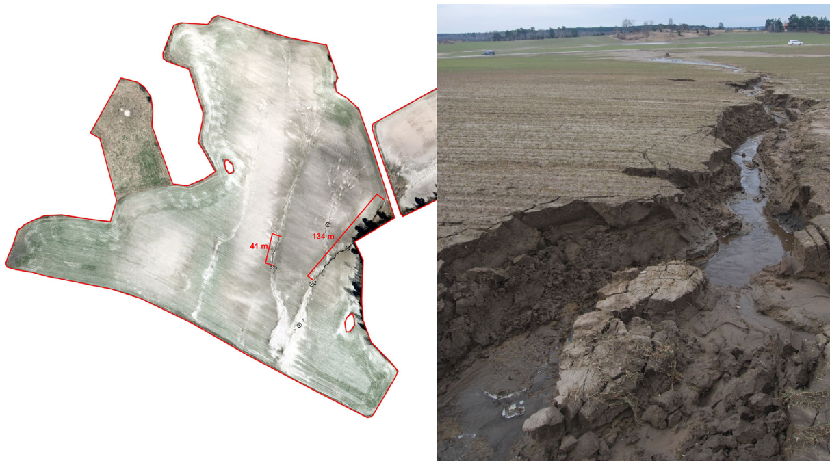
Fig. 4 High-resolution aerial image showing visible erosion gullies in an erosion-susceptible field in the Krusenberg catchment and the positions of soil sampling points ( crossed circles, left ) and an image of a gully observed in April 2013 ( right )
