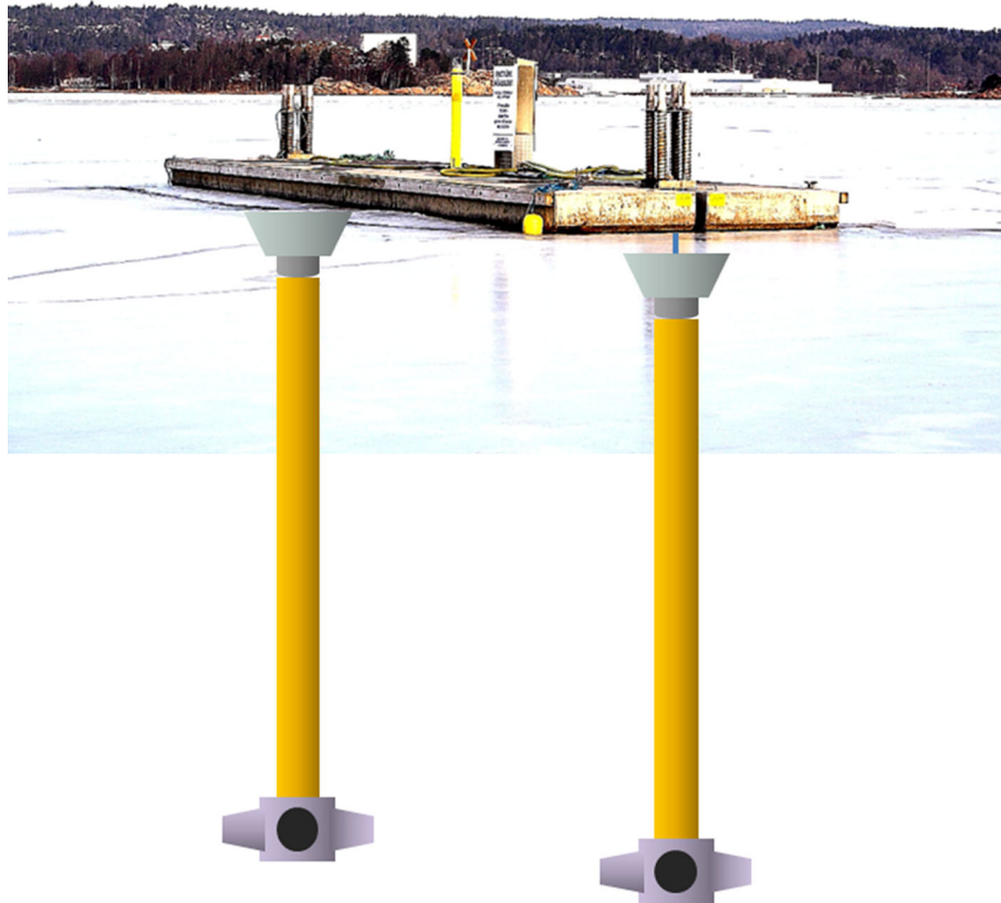
Fig. 2 The pumps hang inside the intake cones in feather clutches below a floating concrete jetty and the nozzles hang in fabric pipes
