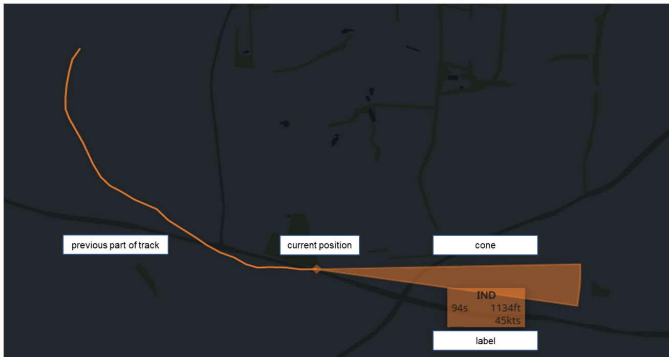
Fig. 3 Wildlife target with expanded extra information on the airside situation display
