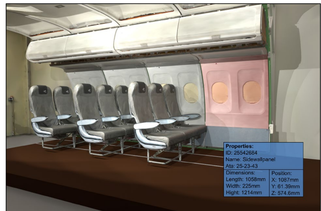
Fig. 11 Example of information stored in a QR-code on a highlighted sidewall panel
