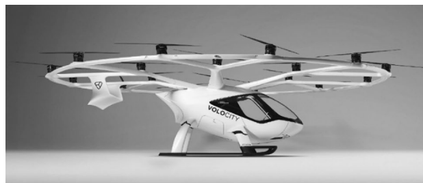
Fig. 3 VoloCity with two seats and 11.3 m maximum vehicle dimension (picture taken from 2021 Volocopter white paper [29])
