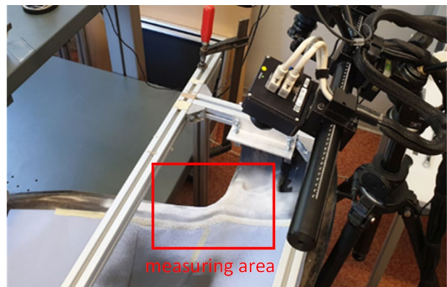
Fig. 13 Detection of surface displacements with an optical 3D measuring system ARAMIS
