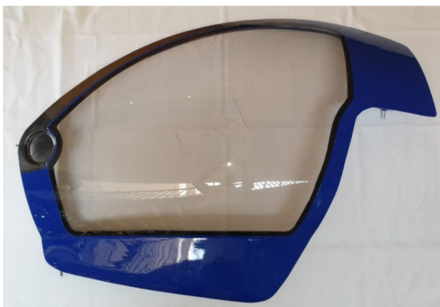
Fig. 11 Front side of bio-based cabin door (partially painted blue for demonstration purposes)
