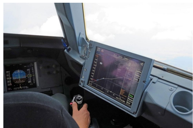
Fig. 6 LNAS displays the optimum vertical profile and the optimum timing of the aircraft configuration changes to the pilots on an electronic flight bag
