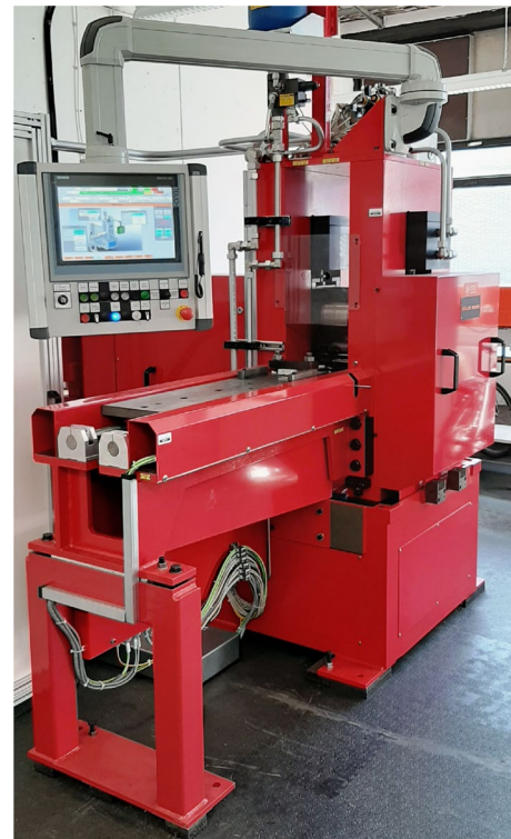
Fig. 3 400 kN cold rolling mill with hydraulically operated pull out table
