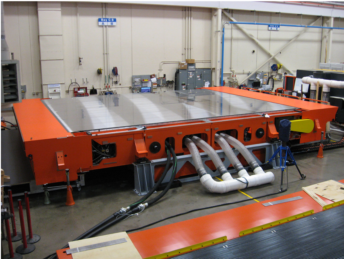
Fig. 6 Moving belt during acceptance testing at MTS
