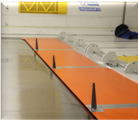
Fig. 8 Boundary layer pressure rakes (left), flying pressure tube (right)
