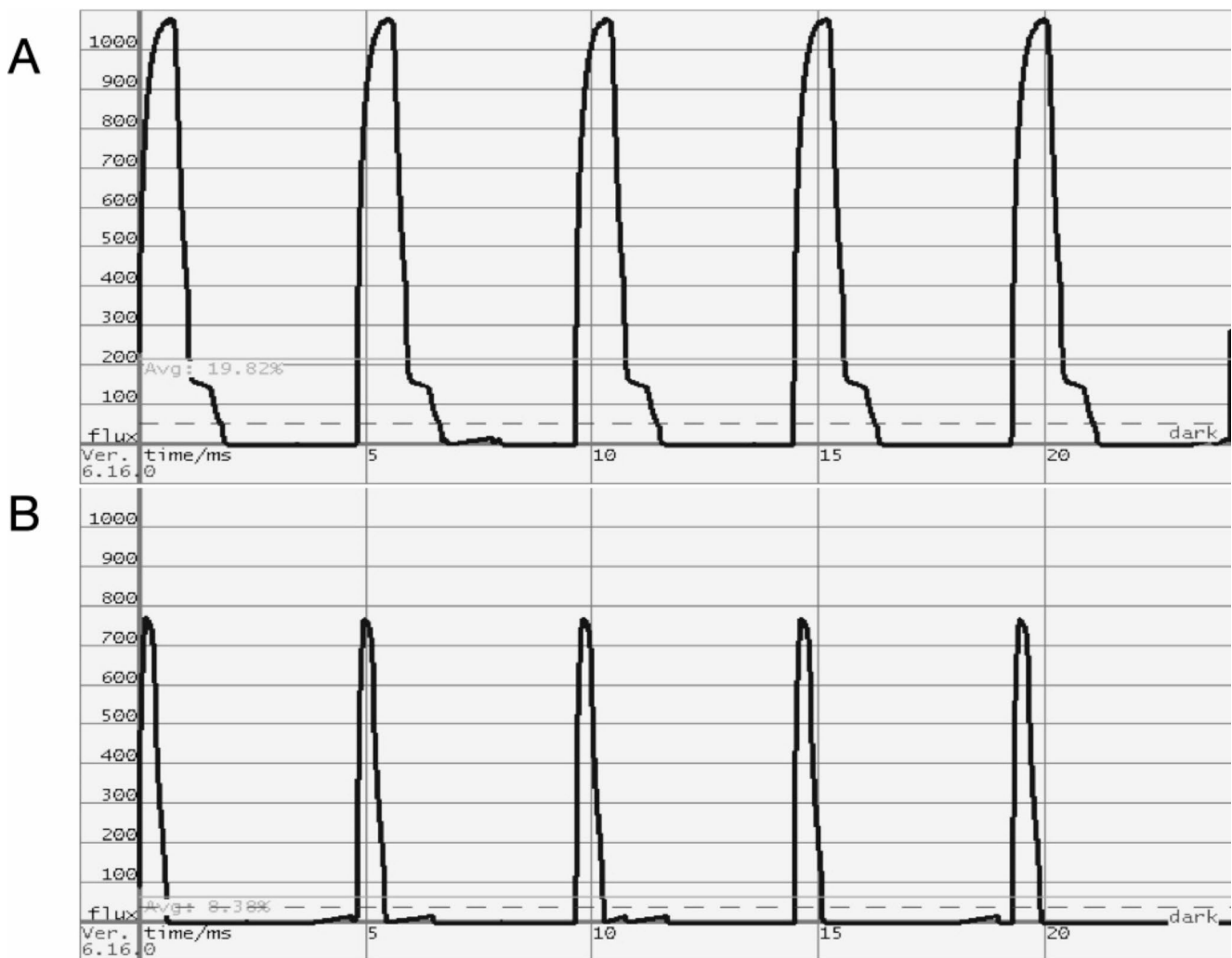
Fig. 1 Light emission of the Dräger Variolux® (Drägerwerk AG & Co, Lübeck, Germany) in non-dimmed (A) and maximum dimmed (B) condition. Light emission over time was 37% in non-dimmed mode and 13% fully dimmed mode
