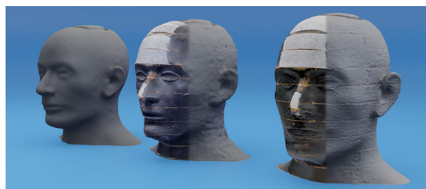
Fig. 1. Comparison of 3D models of the Rando anthropomorphic phantom acquired using Left – CT, Middle – Lidar and Right – Photogrammetry.
