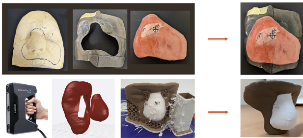
Fig. 2. Comparison of traditional versus additive manufacturing production of combined bolus and shielding devices.
