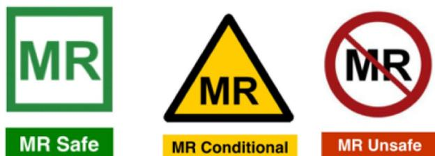
**Fig. 5** ASTM [52] Standard coloured icons for MR compatibility labelling
