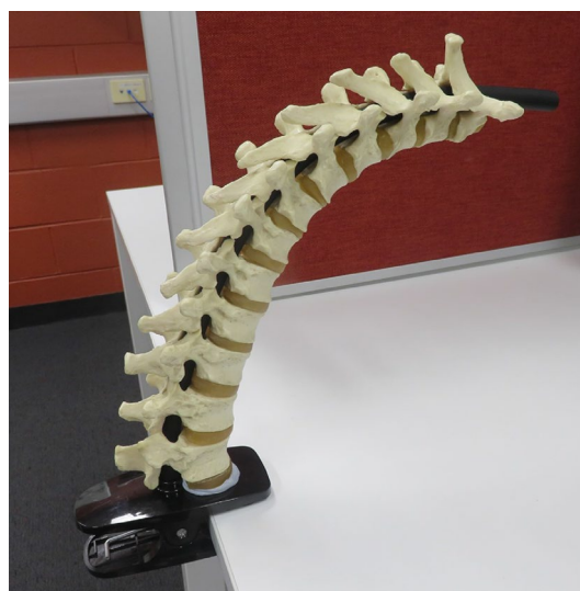
Fig. 1 The phantom spine model (T1–T12) with a flexible rod inserted through the spinal canal
