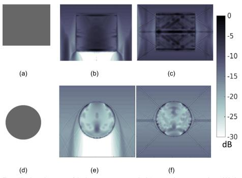
Fig. 3 The ultrasonic coverage of simple components was examined. Image (a) shows a rectangular steel block and images (b) and (c) show the maximum pressure measured at each point in the domain for the limited and full apertures respectively. Image (d) shows a steel disc and images (e) and (f) show the maximum pressure measured at each point in the domain for the limited and full apertures respectively
