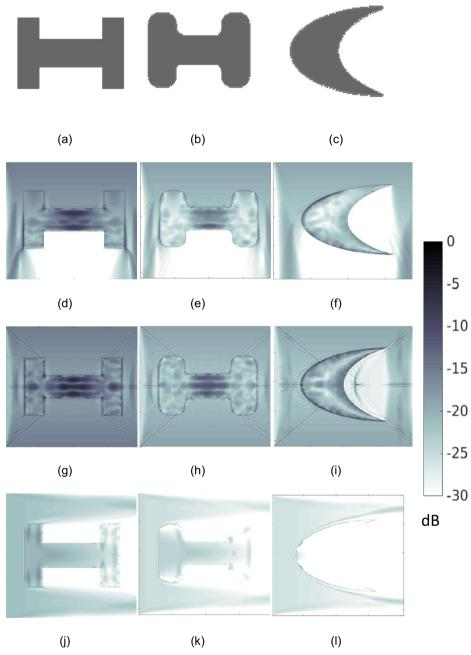
Fig. 4 Images (a-c) show the irregularly shaped components input into the finite element (PZFlex) inspection simulation. Images (d-f) plot the maximum pressure at each point in the domain for a single-sided inspection where the incident plane wave is released at the top of the domain, (g-i) for the full aperture inspection and (j-l) for the single sided inspection where the incident wave travels from left to right
