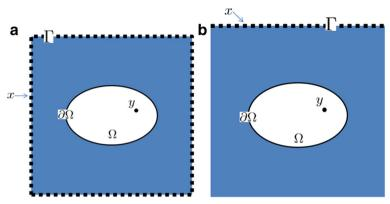
**Fig. 2** Two different inspection scenarios where the dotted line represents the distribution of ultrasonic sources: (a) is referred to as a full aperture inspection and (b) is referred to as a limited aperture or single sided inspection
