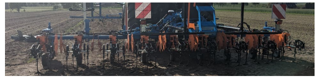
(a) The selective hoe with single coulters actuation.
