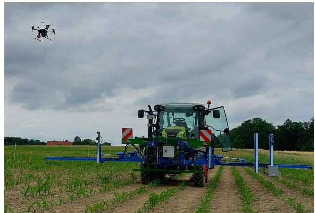
Fig. 3 Ground based sensor mounted on the sensor carrier in front of a tractor and UAV with multispectral camera during data acquisition on 19th of June 2023
