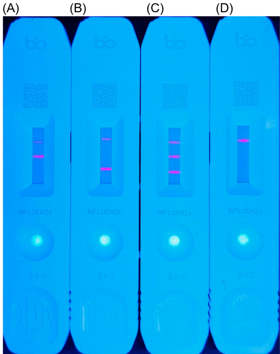
Fig. 3 Fluorescent image of the QuantumPACK Easy Influenza. A Influenza A positive and influenza B negative. B Influenza A negative and influenza B positive. C Influenza A and B positive. D Influenza A and B negative
