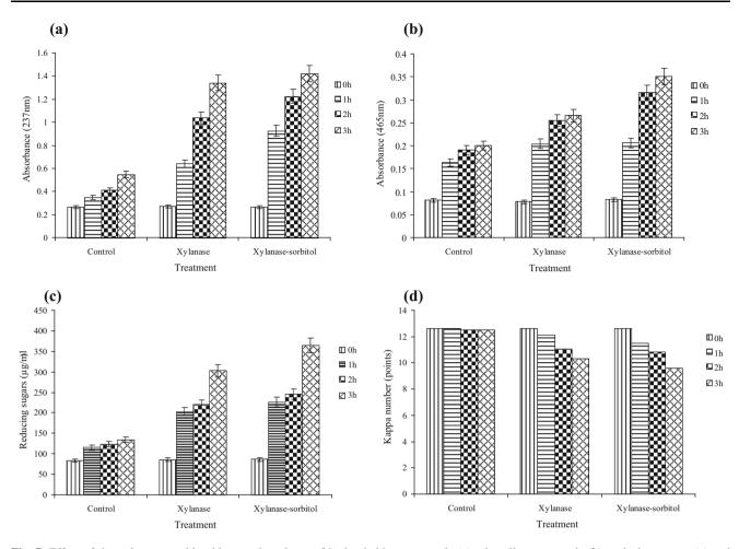
Fig. 7 Effect of the xylanase pre-bleaching on the release of hydrophobic compounds (a), phenolic compounds (b), reducing sugars (c) and kappa number reduction (d) of kraft pulp. Experiments were performed in triplicate and results are mean  $\pm$  SD of three values
