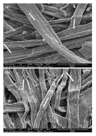
Fig. 8 SEM images of the untreated (a) and xylanase treated (b) pulp fiber at  $\times 1000$  magnification
