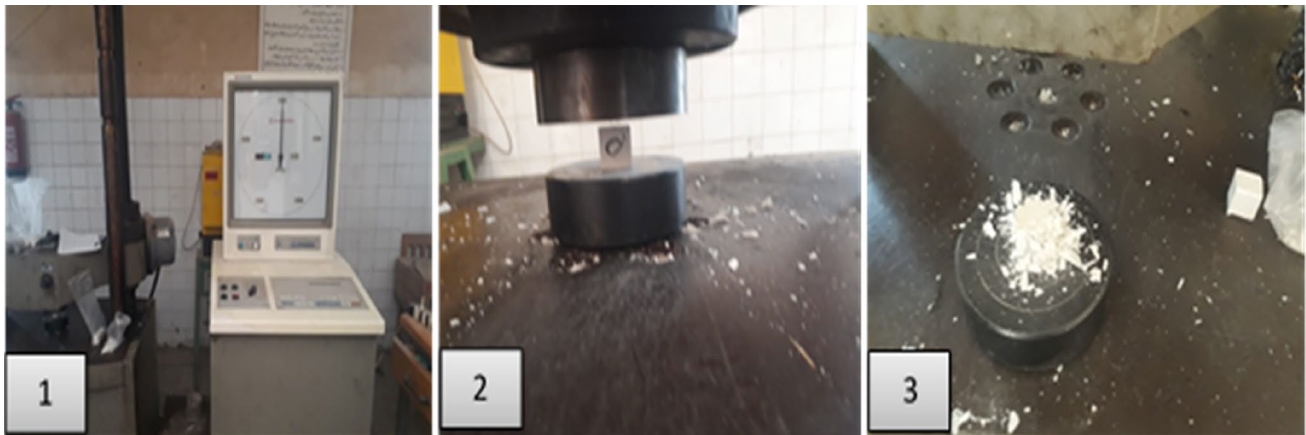
Fig. 9 The compressive strength test on Shemizitu Machine
