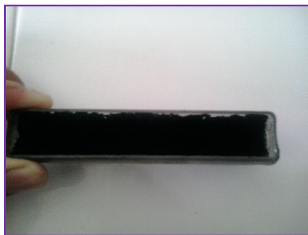
Fig. 4 Optical image of as-grown c-CNTs
