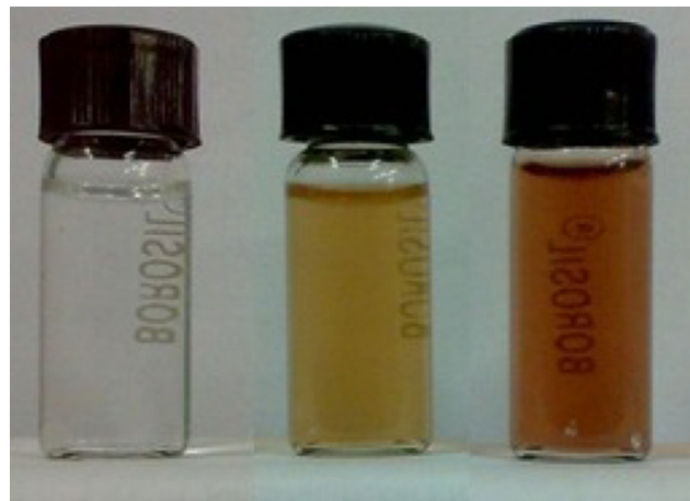
Fig. 1 The aqueous extract of H. musciformis before and after synthesis of AgNPs
