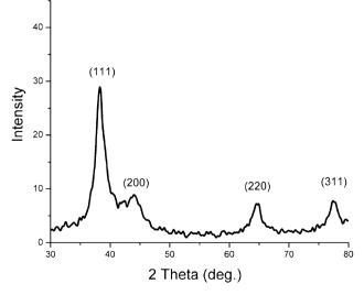
Fig. 5 Typical XRD pattern of the silver nanoparticles stabilized in chitosan
