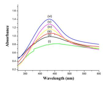
**Fig. 3** UV–visible absorption spectra of silver nanoparticles stabilized in chitosan by varying the time: (*i*) 10 min, (*ii*) 20 min, (*iii*) 30 min, (*iv*) 40 min, (v) 50 min and (v) 60 min
