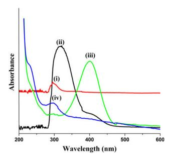
**Fig. 7** UV–visible absorption spectra of aqueous solutions of *(i)* pure 4-aminophenol, *(ii)* pure 4-nitrophenol, *(iii)* 4-nitrophenolate ion and *(iv)* silver nanoparticles catalyzed product
