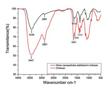
Fig. 4 FTIR spectra of silver nanoparticles stabilized in chitosan and pure chitosan
