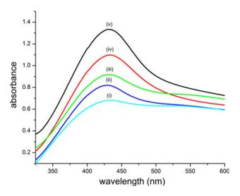
**Fig. 1** UV–visible absorption spectra of silver nanoparticles stabilized in chitosan using various concentrations of (*i*) silver nitrate (0.1 %), (*ii*) silver nitrate (0.2 %), (*iii*) silver nitrate (0.3 %), (*iv*) silver nitrate (0.4 %) and (*v*) silver nitrate (0.5 %) at chitosan (0.5 %) and 50 min of autoclaving
