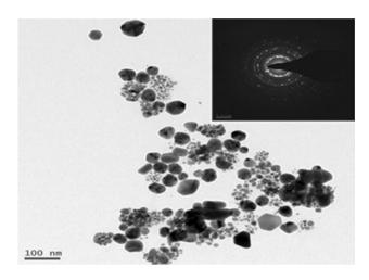
Fig. 6 Typical TEM image of silver nanoparticles in stabilized in chitosan. *Inset* shows the SAED pattern of the silver nanoparticles
