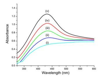
**Fig. 2** UV–visible absorption spectra of silver nanoparticles stabilized in chitosan using various concentrations of (*i*) chitosan (0.1 %), (*ii*) chitosan (0.2 %), (*iii*) chitosan (0.3 %), (*iv*) chitosan (0.4 %) and (*v*) chitosan (0.5 %) at silver nitrate (0.5 %) and 50 min of autoclaving
