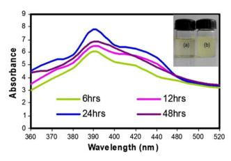
**Fig. 1** UV–Vis absorption spectrum of zinc sulfide nanoparticle. *Inset* **a** shows test tube containing the culture supernatant of *S. nematodiphila*, **b** *S. nematodiphila* biomass with zinc sulfate
