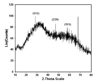
Fig. 2 XRD pattern of zinc sulfide nanoparticle
