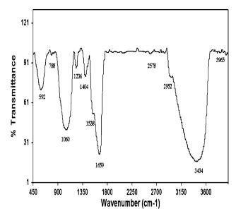
Fig. 6 FTIR spectrum of zinc sulfide nanoparticle synthesized by using S. nematodiphila
