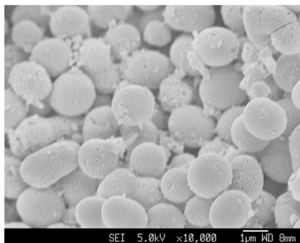
Fig. 3 A FESEM image of 1 \mu\text{m} sized ZnO spheres obtained with \text{Zn}(\text{NO}_3)_2 \cdot 6\text{H}_2\text{O} concentration of 0.1 mol/l
