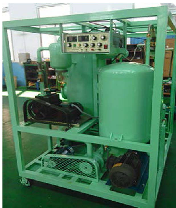
Fig. 3 The experimental setup for conducting the demulsification experiment of W/O emulsion
