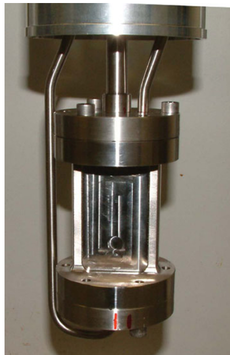
Fig. 5 The GEM diffractometer high temperature gas flow cell, capable of up to 1,300 K and a variety of atmospheres and gas flow rates
