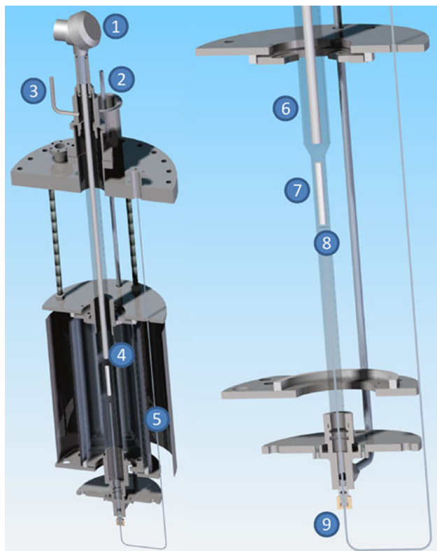
Fig. 4 The schematic diagram of the flow-through gas cell (with the right hand portion highlighting the central portion of the left hand figure), showing (1) oxygen and temperature sensor; (2) gas inlet; (3) gas outlet; (4) heater element; (5) heat shielding; (6) quartz sample holder; (7) sample; (8) quartz frit; (9) thermocouple, from [10]
