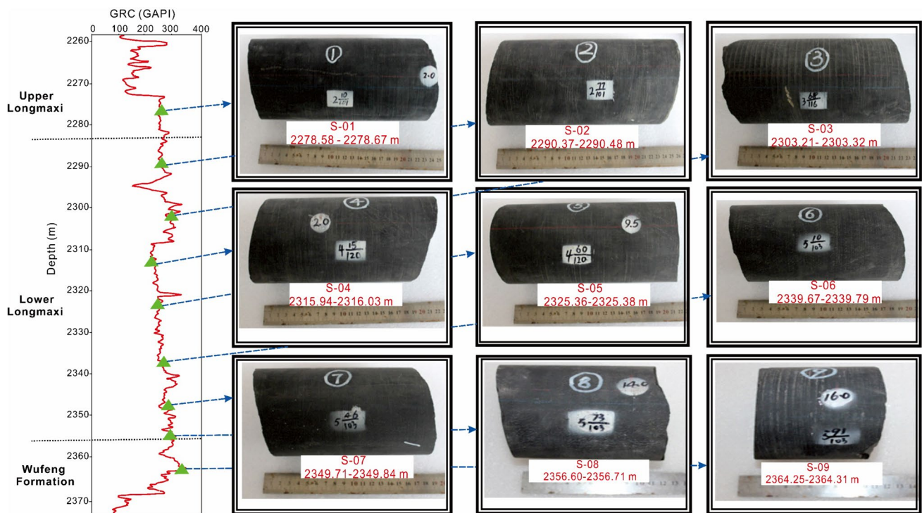
Fig. 2 Core samples from well JY-1X before geomechanical tests. On the gamma-ray log curve (left), sample depths are highlighted with green triangles. The representative cores numbered from S-01 to S-09 (right) correspond to sublayers 9# to 1# according to sample depths
