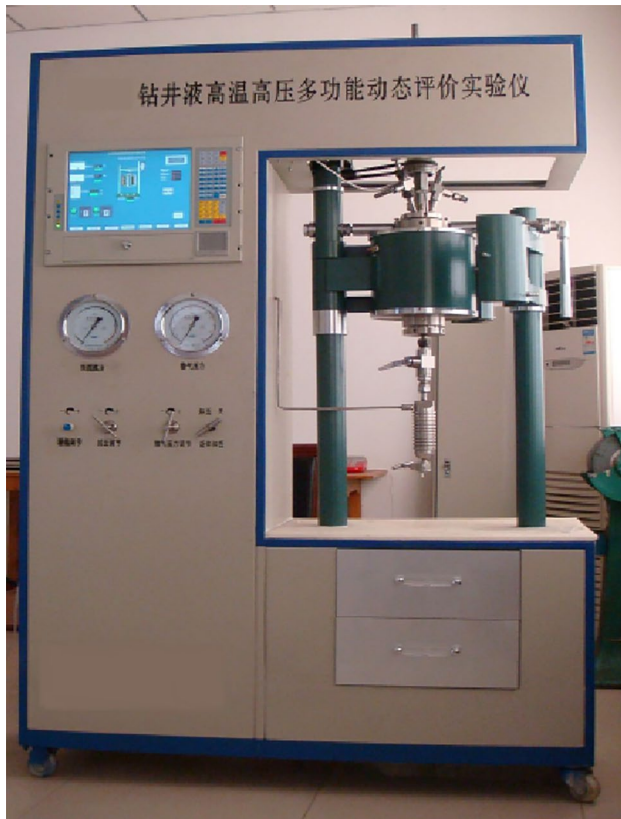
Fig. 1 High-temperature and high-pressure multi-functional dynamic filtration for drilling fluid
