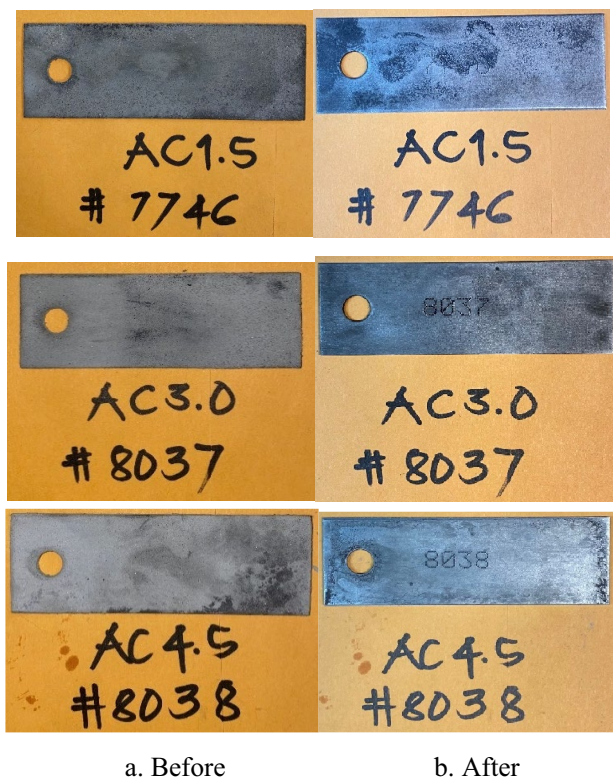
Fig. 5 Corrosion plates in potassium chloride (KCl)
