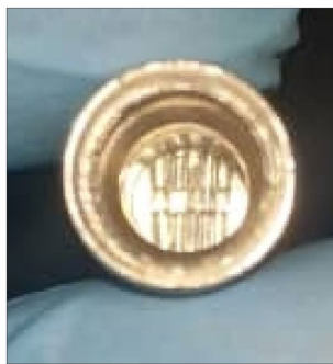
Fig. 3 Capillary Tubes containing sample placed inside the HP-μDSC cell
